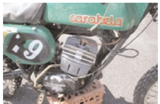
The aluminum parts show plenty of corrosion from outdoor exposure.
