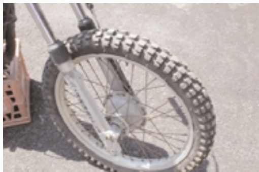
The finish on the forks is also flaking from outdoor exposure.
