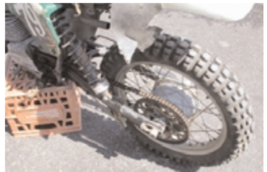
The shocks are rusted and seized.
